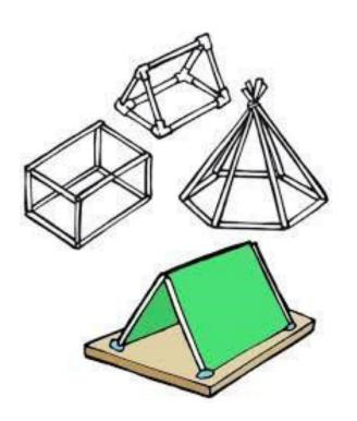
A frame structure is made up of a rigid arrangement of parts, or structural components, fastened together.
